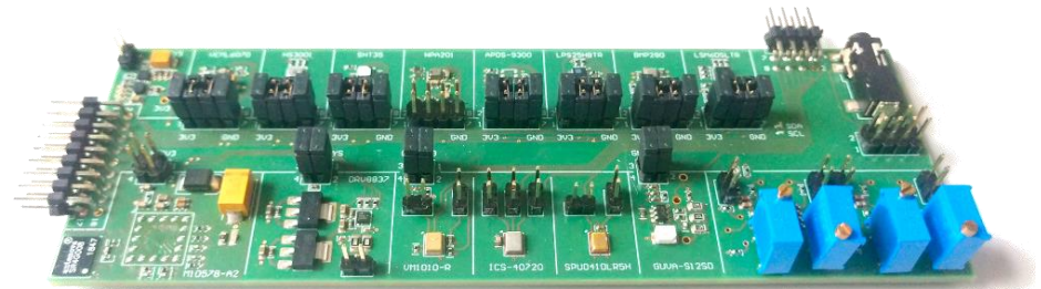
Test board with pre-selected sensors
